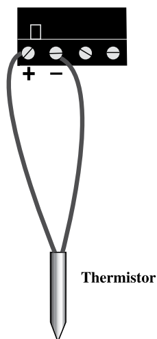
Wiring a Temperature Sensor
